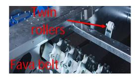
7) Low maintenance: Under all type of carpets there are some rollers that support the belt. After some years the bearings of the rollers may be subject to seizure; but they are under the carpet and it is difficult that the operator notices immediately with consequent consumption of the belt. FAVA install in his carpet a twin rollers obtaining a redudant system that means less maintenance. In the rubber belt that is no possible.
