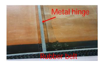
5) <u>Draining surface</u>: plastic belt has a draining surface because there is a lot of guides under the carpet and low friction (look the picture). Otherwise the rubber belt crawls on a metal sheet and if some water enters between the carpet and the metal sheet it can form a layer of ice that can block the belt. High contact area between rubber belt and metal sheet leads high friction.
