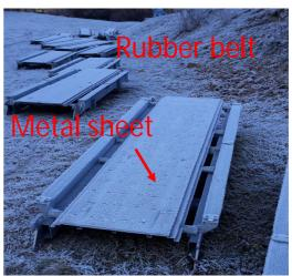
5) Unslippery surface: Fava belt has a new type of unslippery rubber pad made from a soft mix for a great grip (tested with slope more of 30%). This pad has a vulcanized washer inside and it can't go out from his housing cavity. Otherwise the rubber belt is slippery because has a small contact area between skiers and carpets (look the picture).
