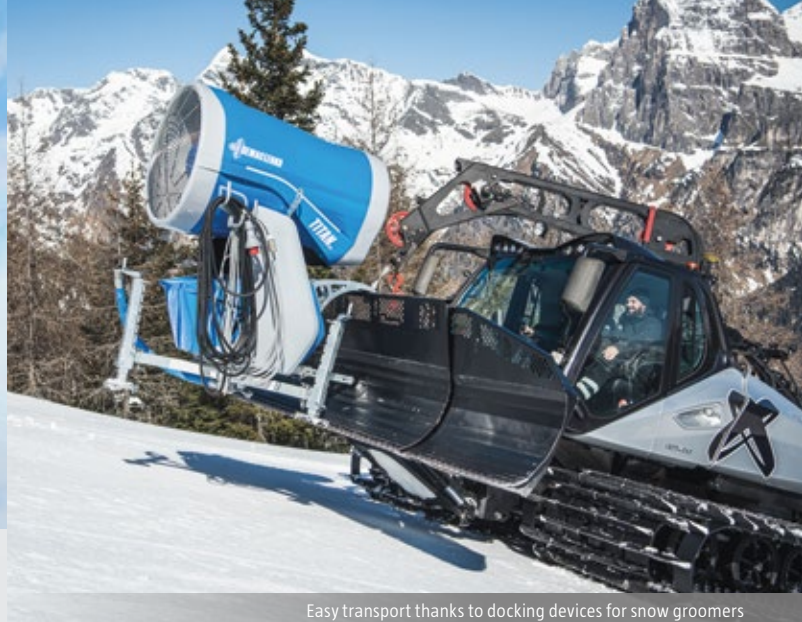
Easy transport thanks to docking devices for snow groomers
